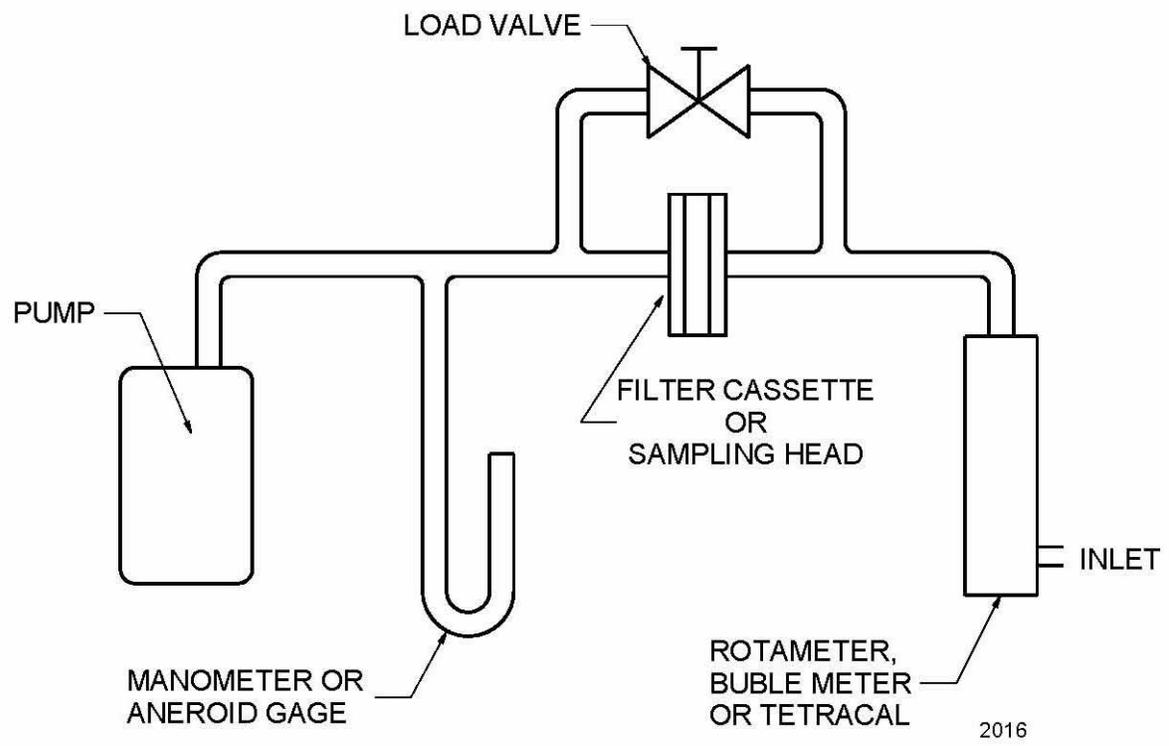
Figure 1: Schematic of Flow Setting and Testing Circuit
