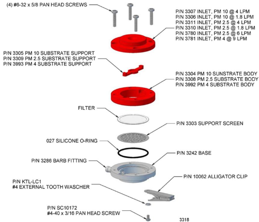
**Figure 3. Exploded View of H-PEM**
