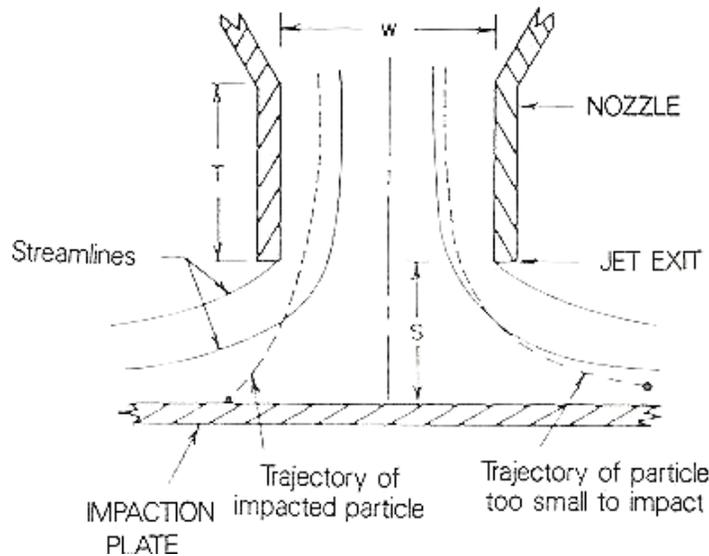
**Figure 2. Schematic Diagram of a Typical Impactation stage Showing Streamlines and Particle Trajectories (after Marple et. al.)<sup>4</sup>**
