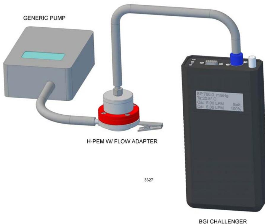
**Figure 4. Schematic Diagram of Typical Calibration Arrangement.**
