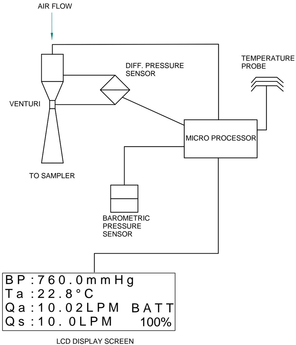
Figure 4 – Schematic Diagram of tetraCal®
