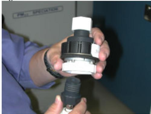
Figure 3 -21: Attach the TriCAL to the audit adapter.
