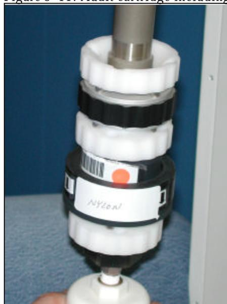
**Note: Use these cassette assemblies for leak checks and flow rate audits only.**
