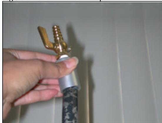
Figure 3 -14: Close valve lever for leak check.
